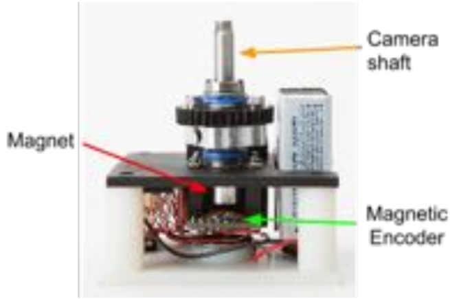
Figure 13a: Encoder mechanism
