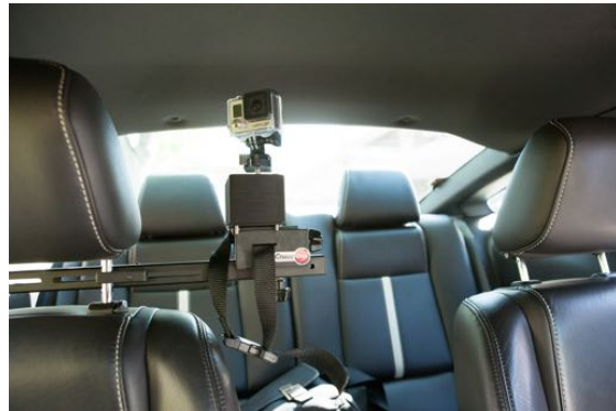
Figure 2: Video mount on headrest
