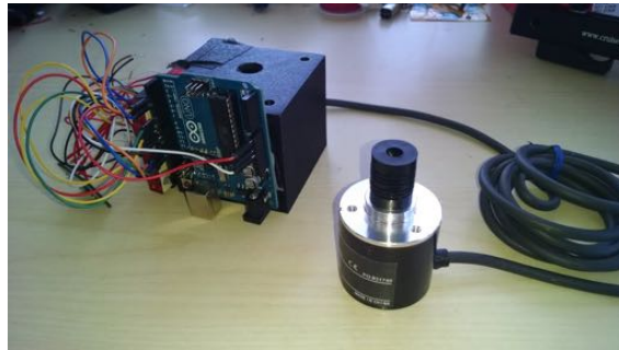
Figure 20: Optical encoder controlled mount
