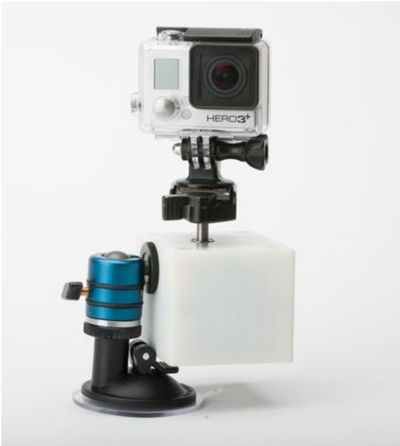
Figure 12: Final product with GoPro and suction cup attached
